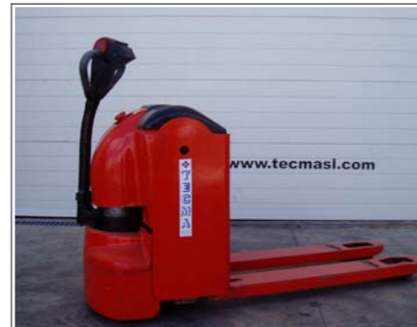
TP electrica - YALE MP22
